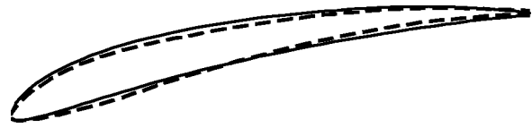
Fig. 3 Influence of moment of inertia on resulting profiles (dashed line: original; solid line: cross section area and moment of inertia taken into account)
